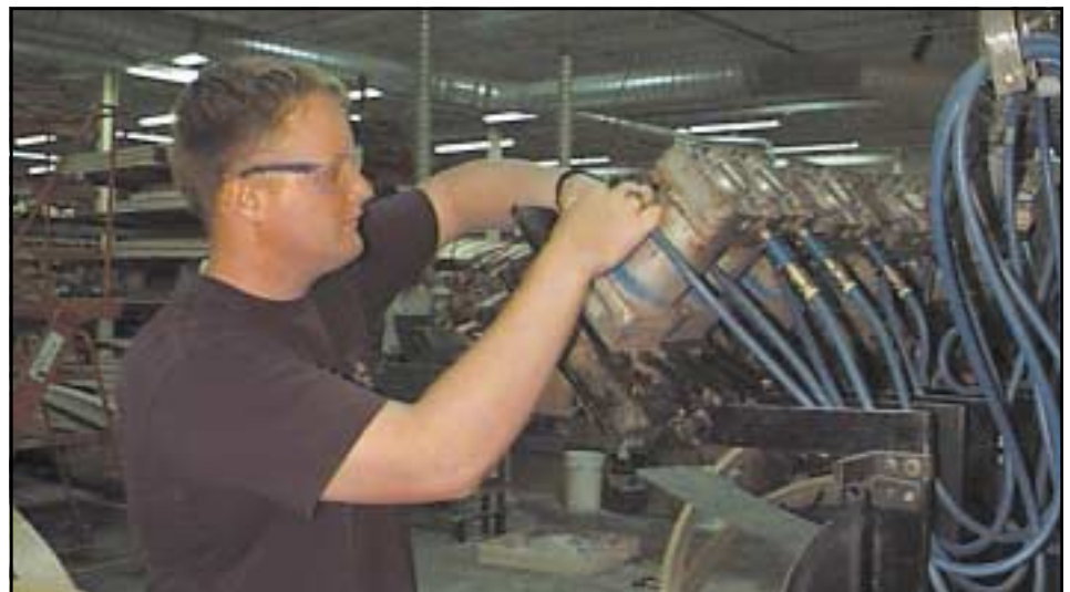
Randy Martens repairs leaky compressed air fittings on a radius clamp used to manufacture Loewen's line of arched windows.
